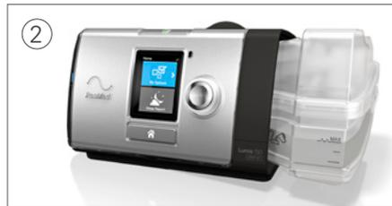
Close the humidifier and insert it into the side of the device.
