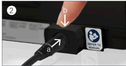
(a) Plug the power connector into the device power inlet then (b) push down the retention clip to secure in place.
