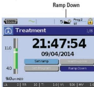
If you experience difficulties in taking off the ventilation, you can use the Ramp Down feature. This feature reduces the treatment pressure to Start EPAP/PEEP over five minutes. After five minutes the therapy stops. You can enable the Ramp Down feature when it is selected by the physician in the Options menu.
