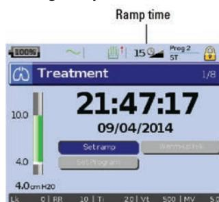
Ramp time is a feature that can be enabled by your clinician by setting a maximum ramp time. Designed to make the beginning of treatment more comfortable, ramp time is the period during which the pressure increases from a low start pressure to the treatment pressure. Refer to Setup menu: Options (see page 14).
