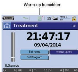
Check that the warm-up feature is displayed on the **Treatment** screen. Start the warm-up feature. Check that the humidifier warm-up symbol is displayed on top of the screen.
