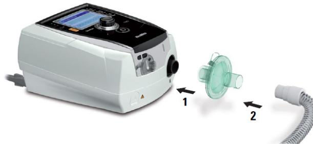
1. Fit the bacterial/viral filter to the air outlet of the device.
