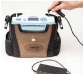
1 To charge the internal battery, connect the AC power supply to the device and plug it into an electrical socket. A plug icon
