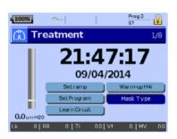
Selecting the mask type and performing a Learn circuit enables to calculate the impedance and leak for controlled therapy pressure. See "Setup menu: Options" on page 45.
