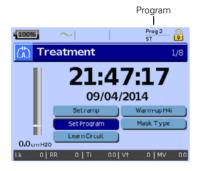
Up to two sets of therapy settings (Programs) can be saved for different device configurations (eg, individual Learn Circuit results) in addition to ventilation and alarm settings. They are stored while in the *Clinical Settings* menu. If both, ie, dual, is selected, the patient can choose the program to use on the *Treatment* screen. If only a single program is selected, the option does not display.
