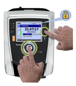
To activate Clinical mode ①, hold down and simultaneously for at least three seconds. You will be prompted for how long the device should stay in this mode. After the set period of inactivity or next power cycle (power on/off), the device automatically switches back to the patient mode and the device beeps.
